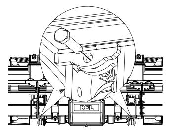
Image 29. The tilt linkages' transport protection.
