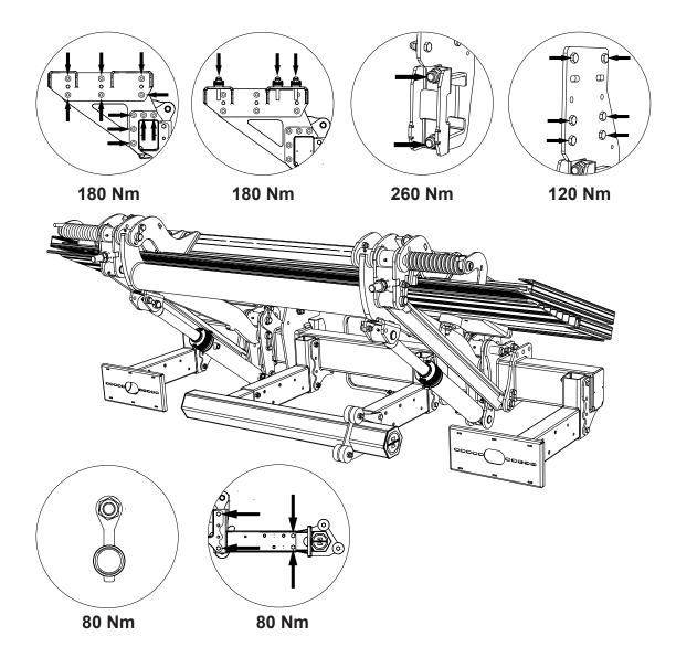
Image 61. Tightening torque
