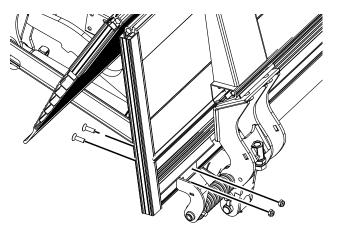
Image 23. Refit the auxiliary spring brackets.
