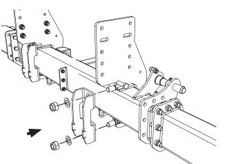
Image 10. Install the U-profile with associated washers and nuts, but do not tighten these.
