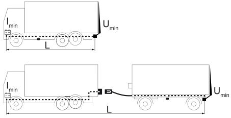
Image 59. Maximum power consumption - Minimum recommended conductor cross sectional area
