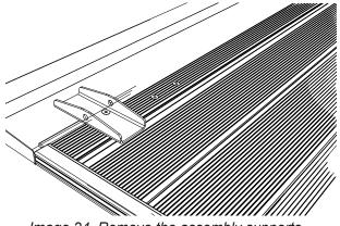
Image 24. Remove the assembly supports.
