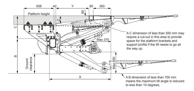
Lifting height: 920 - 1350 mm. Ensure sufficient ground clearance is obtained.
