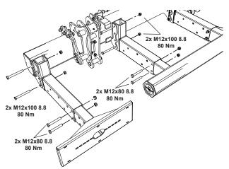
Image 36. Installing underrun protection
