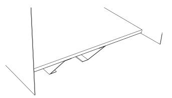
Image 7. Make a cut-out in the floor of the body.
