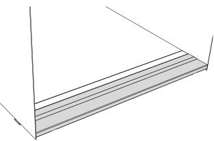
Image 9. Align and securely weld the floor extension to the previously installed steel section.
