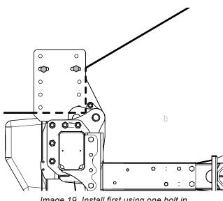
Image 19. Install first using one bolt in the bracket's slot-shaped holes.
