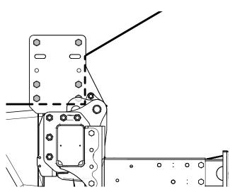
Image 21. Install the chassis bracket with at least six M14x45 10.9 bolts.
