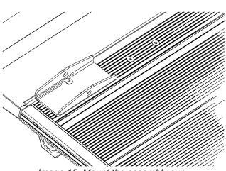
Image 15. Mount the assembly supports using one bolt each.
