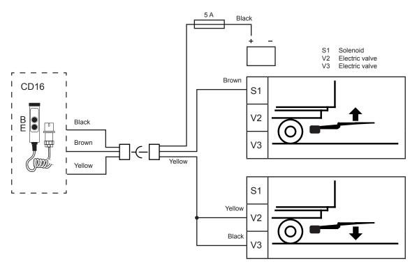
Image 44. Lift with one control device.
