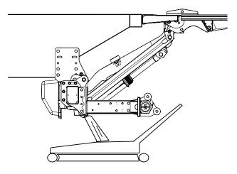
Image 17. Tighten the bolts and hang the platform onto the floor extension by means of the assembly supports.
