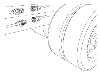
Image 30. Quick connectors must be well protected.
