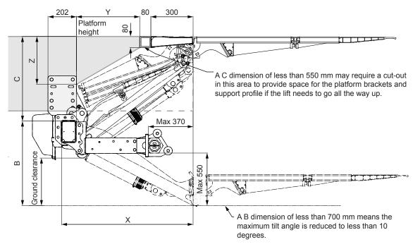
Lifting height: 1013 - 1350 mm. Where lifting height is less than 1060 mm, consider a shorter platform!
