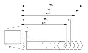
Image 35. The outer part of the brackets can be fitted in one of five positions
