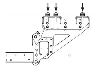
Image 25. Fit the support frame to the trailer chassis using the clamps.
