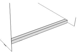
Image 8. Reinforce the edge of the floor where the floor extension is to be installed with a suitable steel section.
