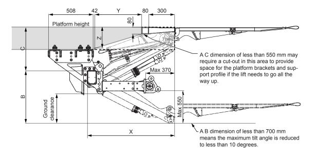
Lifting height: 970 - 1350 mm. Where lifting height is less than 1000 mm, consider a shorter platform!
