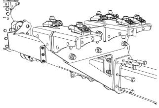
Image 12. Install the brackets on the support frame with its opening facing downwards.
