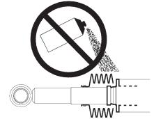
Image 1. Piston rods, cylinder covers and boots must not be painted/coated
