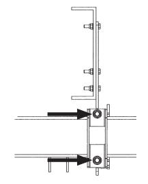
Image 20. Thechassis brackett requires at least 35 mm clearance between vehicle chassis and support frame.
