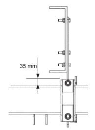
Image 18. The chassis bracket requires at least 35 mm clearance between vehicle chassis and support frame
