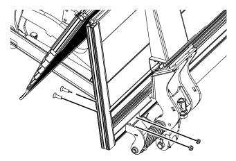
Image 28. Refit the auxiliary spring brackets.
