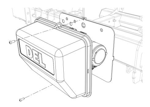
Image 42. The protective cap is secured with two bolts
