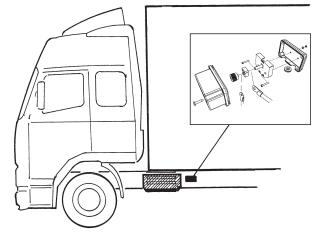
Image 33. The fuse box must be installed in a well protected position as close to the battery as possible
