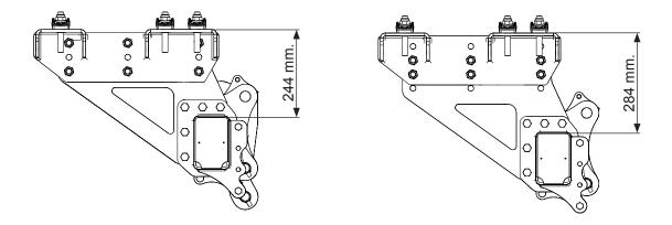
Image 13. Adjustment of the chassis brackets' height.
