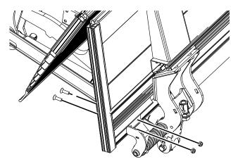
Image 14. Uninstall the auxiliary spring brackets.
