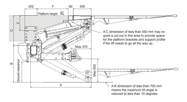
Lifting height: 970 - 1350 mm. Where lifting height is less than 1000 mm, consider a shorter platform!
