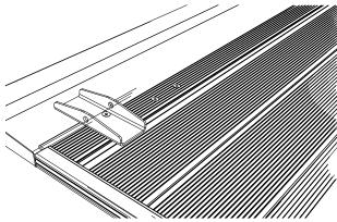
Image 16. Tighten the bolts and hang the platform onto the floor extension by means of the assembly supports.
