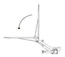
To adjust the speed for tilt down there is an adjustable constant flow valve on the valve block. see figure below. (The figure shows a valve block for Z, ZHD models)
