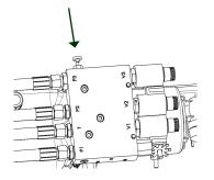
The lowering and lifting speed may not exceed 0.15m per second = 1.5m per 10 seconds.
