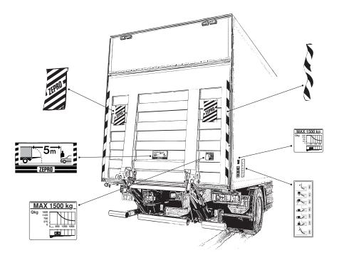
There is a small warning set, spare part number 31290 containing: Decal "Working area" 2pcs Warning flags incl. mounting profile 5m x 50mm Warning tape
