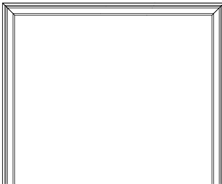
Figure 43. Angled cuts on Top Double Rail and Side Double Rails should make 90° corners.
