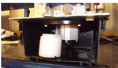
How the filter should be placed inside the tank.
