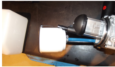
No need to be cut. Just mount the filter on the hose.
