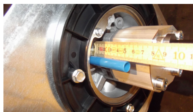
Cut the return hose so it's lenght is 60 mm. 50-52 mm should be left after fastening in to the adapter block.
