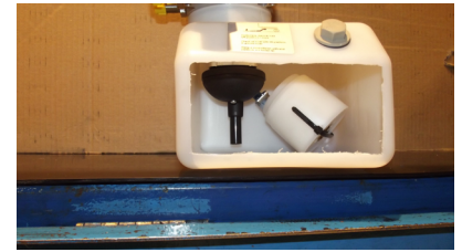
How the filter should be placed inside the tank.
