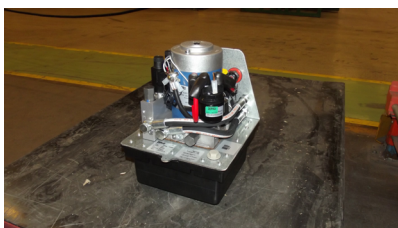
On this model the return hose needs to be cut.
